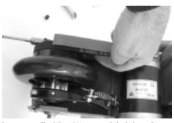
Fig 13 and 14. Tighten both axle adjusters equally, 1/8 to 1/4 turn until the belt or chain is properly tensioned.
